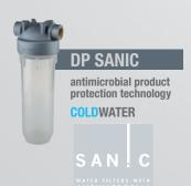
Max working pressure: BSPP versions 8 bar (116 psi). NPT versions 8,6 bar (125 psi). Max working temperature: 45°C (113°F). Materials: Reinforced PP, PET. Accessories:
