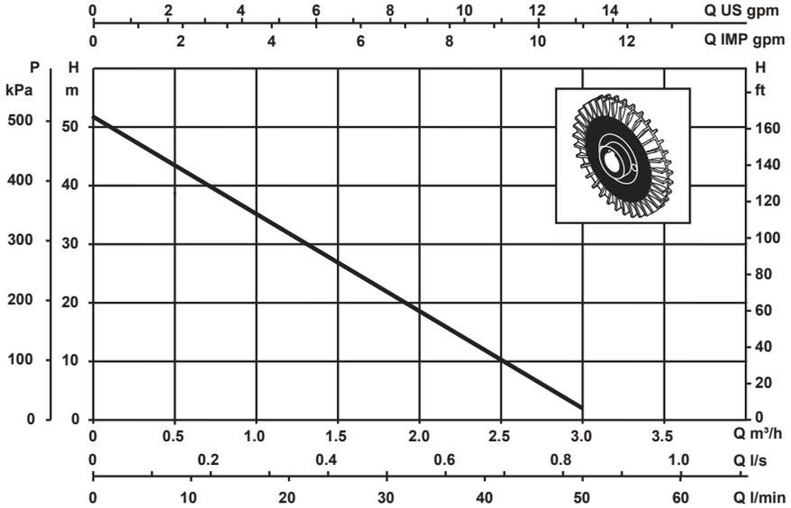
The performance curves are based on the kinematic viscosity values = 1 mm<sup>2</sup>/s and density equal to 1000 kg/m<sup>3</sup>.
