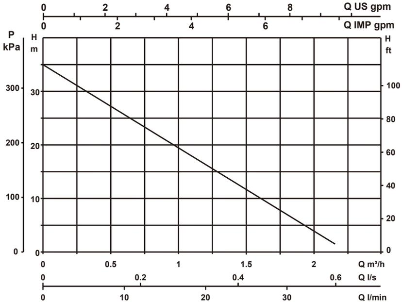
The performance curves are based on the kinematic viscosity values = 1 mm<sup>2</sup>/s and density equal to 1000 kg/m<sup>3</sup>. Curve tolerance according to ISO 9906.
